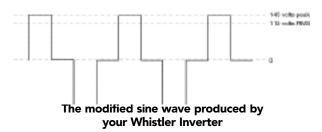
The modified sine wave produced by your Whistler inverter has a root mean square (RMS) voltage of 110 volts. The majority of AC voltmeters are calibrated for RMS voltage and assume that the measured waveform will be a pure sine wave.
